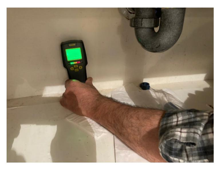
Figure 2 A moisture meter shows over 100% moisture (Red) behind the drywall underneath the Master Bathroom
