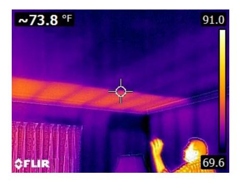
Figure 4 Thermo Image ceiling below bathroom Dark purple detects moisture
