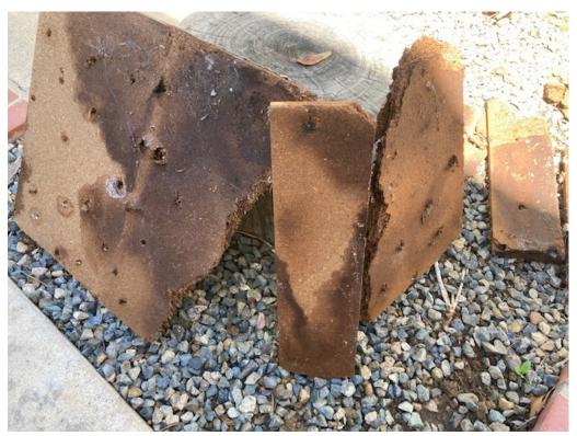
Figure 3 Here is the remains of the fiber board that was removed under the kitchen sink
