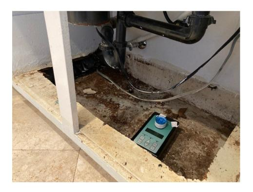
Figure 1 a non-viable air sample was taken underneath the kitchen sink. The air sample revealed toxic mold. ( see findings and recommendations)
